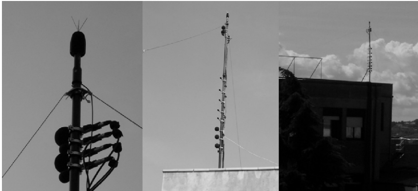
Fig. 7. Experimental setup for outdoor tests, the array was placed at the edge of a terrace high enough with respect to the street and the surrounding buildings to ensure that no urban noise was impinging within the critical angular incidence range. At the top of the array it can be seen the outdoor microphone of the sound level meter.
